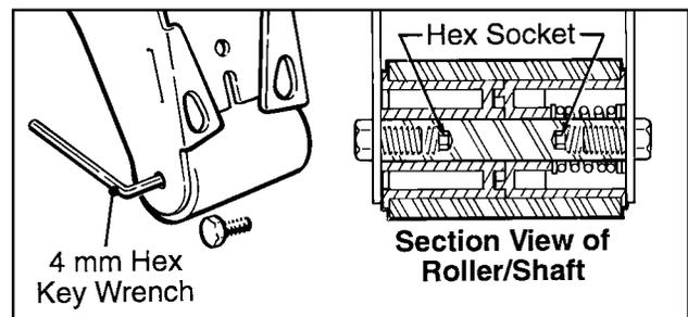
Figure 4-3 – Section View of Roller Shaft
