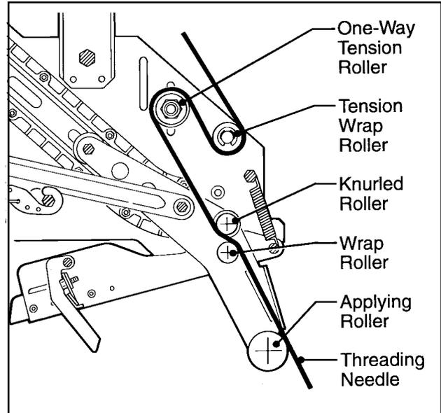
**Figure 3-3 – Tape Loading/Threading**
