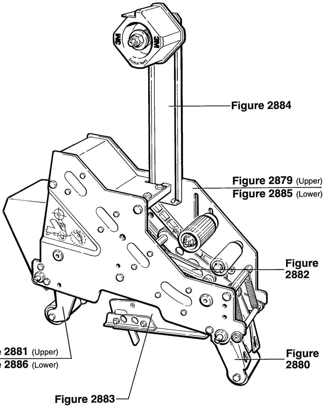
**Taping Head Assemblies – AccuGlide™ II STD 2 Inch**
